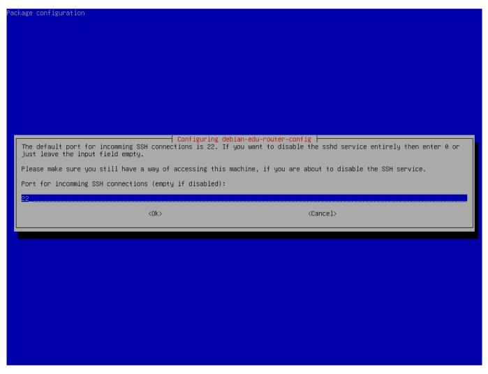
Configure the SSH port, this should be 22 if the configuration has not been changed.
