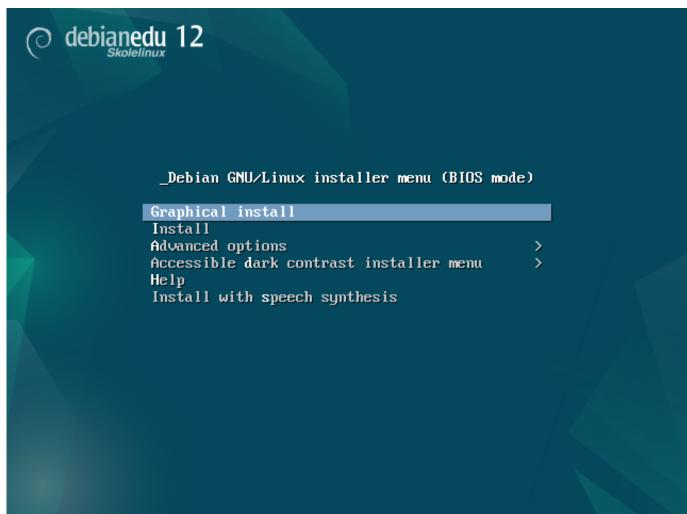
**Graphical install** uses the GTK installer where you can use the mouse.
