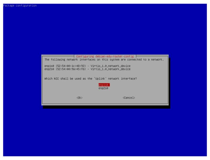
Select the interface which is connected to the upstream network.
