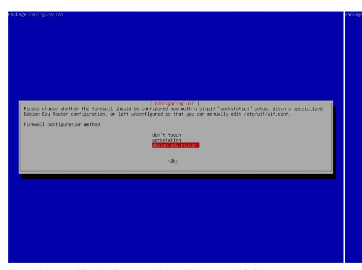
When asked about the uif firewall configuration method choose "debian-edu-router". Confirm that you want to set up the firewall for Debian Edu Router.
