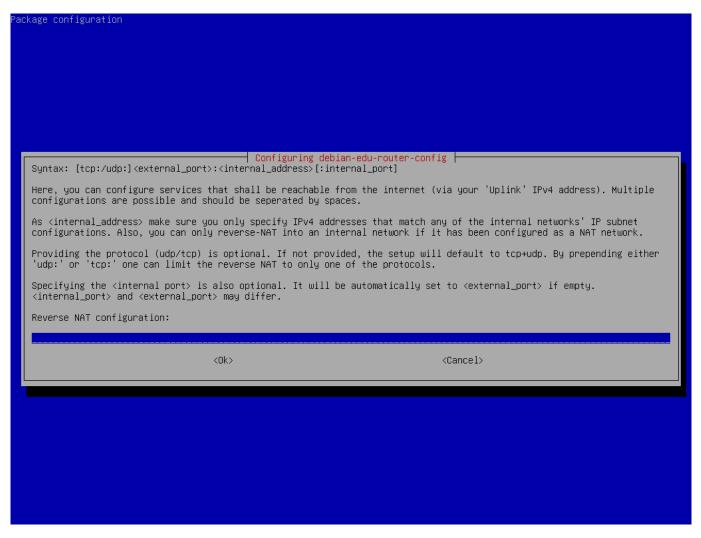
If you want to expose any internal services to the internet you can configure them using the described syntax. Note that SSH access to the gateway can be configured using the following dialog.
