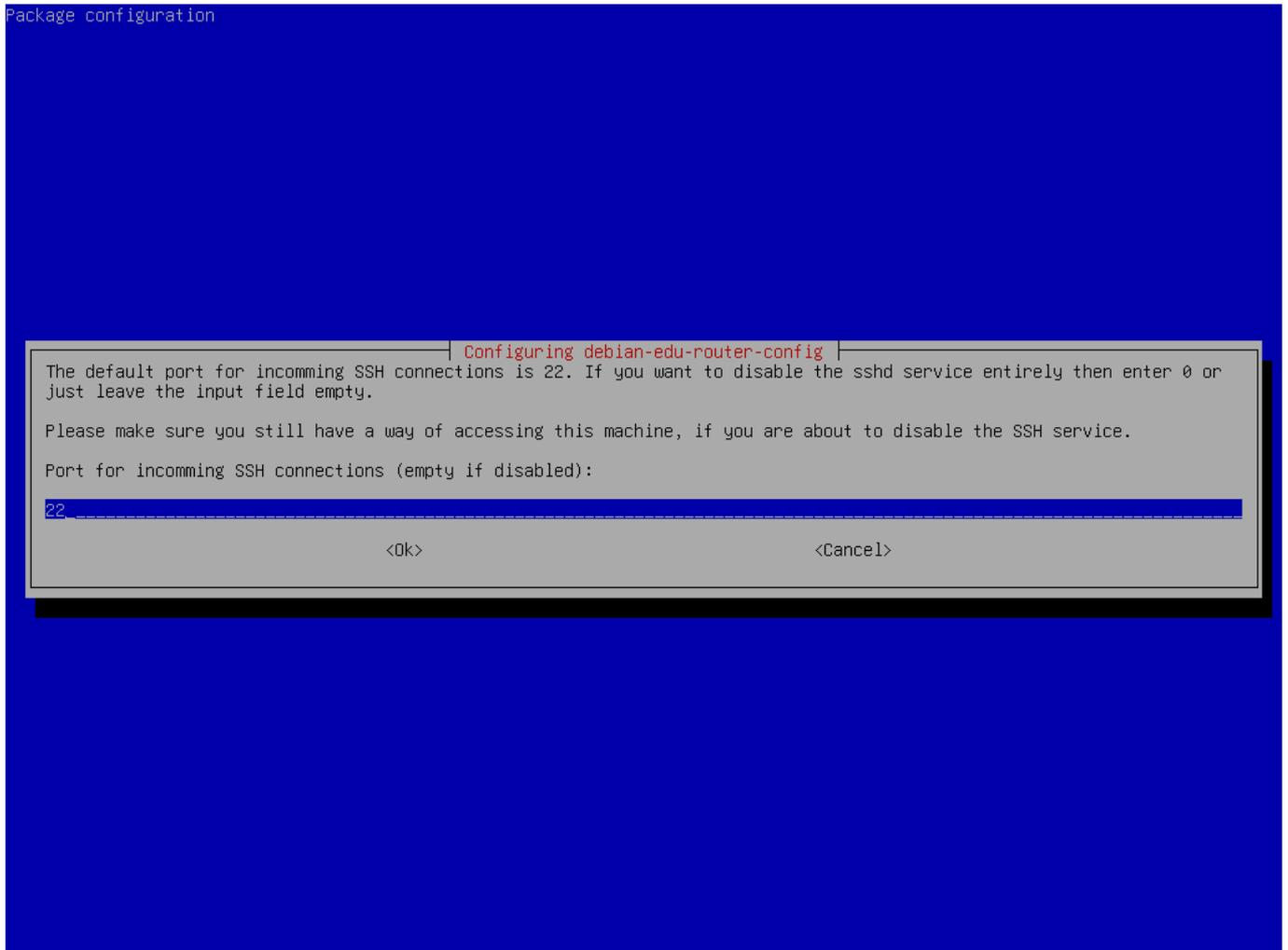
Configure the SSH port, this should be 22 if the configuration has not been changed.
